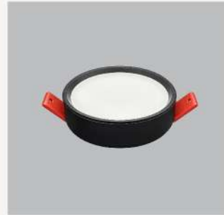
VOL: 85/265 (v) POWER: 2 (w) LUM: 70/130 (lum/w) CCT: 3000 up to 6500 (k) CRI: 85 up to 97 SIZE: 80 mm IP: 20
